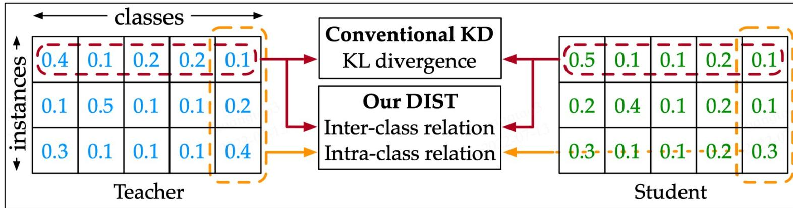
By replacing the original KL divergence with Pearson distance, we have the following KD loss:
